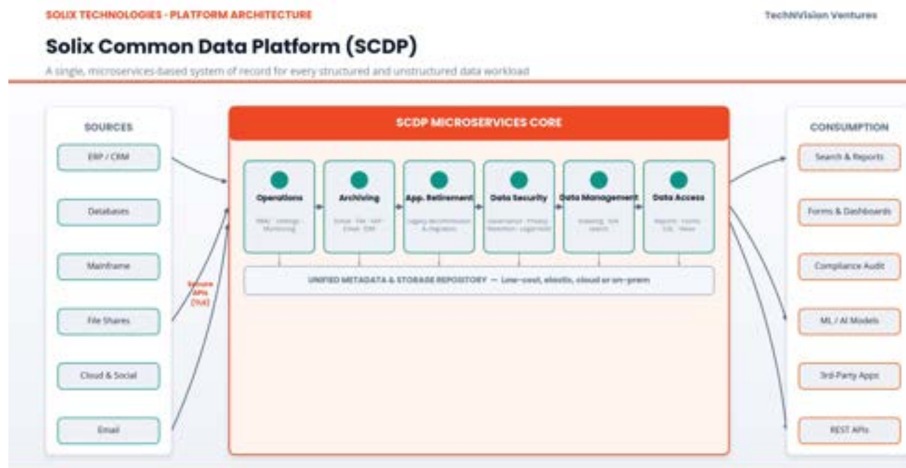
Figure 2. SCDP unified microservices architecture — from source systems to consumption.
